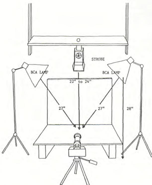
**Figure 2.** The author's set-up for photomicrography. ♦The specimen is placed on the L-shaped stand, at the convergence of the arrows. ♦The strobe is usually positioned above and behind the camera, and may be mounted or hand-held. It may be moved to the left or right to minimize reflections. ♦The BCA lamps are usually positioned above and on both sides of the specimen, with their reflectors aimed so that no direct light hits the camera.
