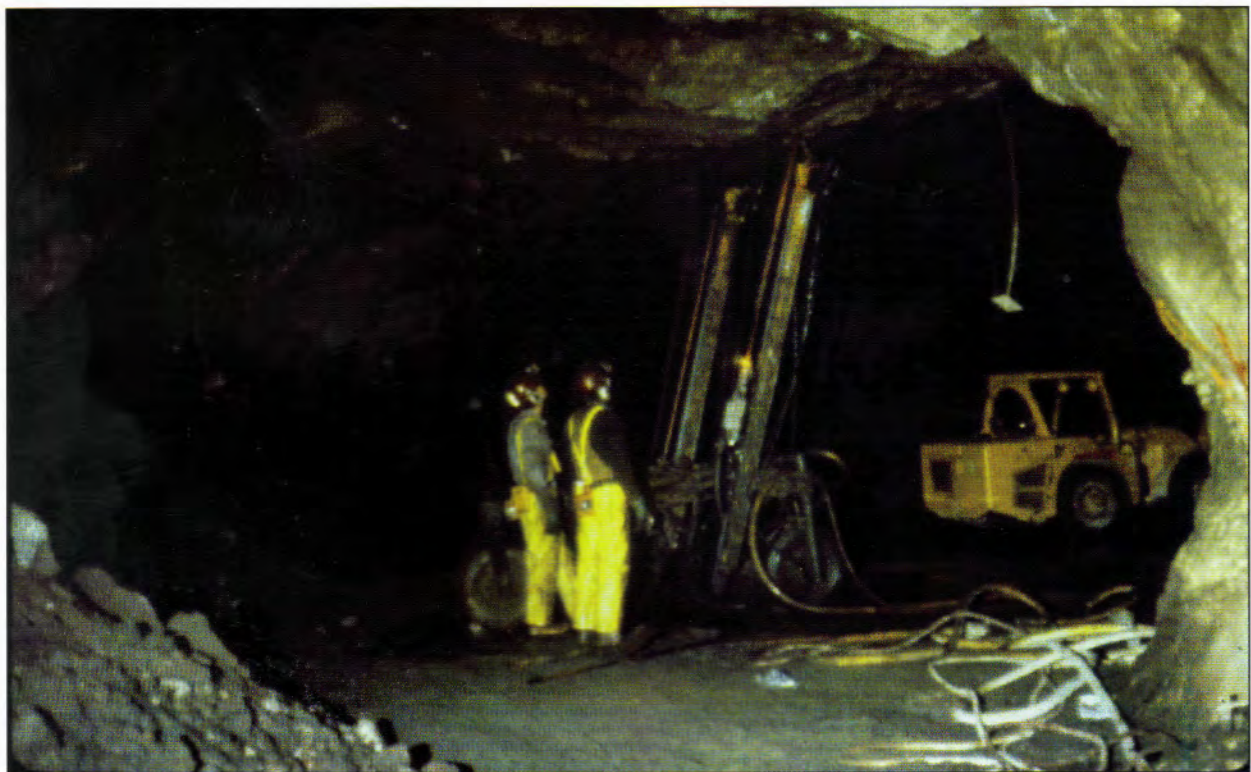
Above: A trammer dumping ore from a rocker-dump car down the ore pass. Sterling Hill, circa 1976. F. Bernard Kozykowski archives photo. Below: Chris Auer and helper, running a “Jumbo” drill in a large Sterling Hill stope, circa 1976. F. Bernard Kozykowski archives photo.
