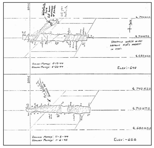
**Figure 2.** Jack Baum surveyed and drew these mine maps in 1944–45 for the New Jersey Zinc Company (NJZ) of the Franklin Mine 710 North top slice, 648 and 658 elevations (i.e., feet below the collar of the Parker Shaft). At a later date, Jack noted on the diagram at the 648 elevation "Wollastonite here. First known occurrence at Franklin," and at the 658 elevation "More wollastonite recovered here."
