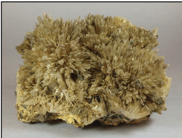
Figure 8. Intergrown radiating aggregates of translucent, pale brown, spiky aragonite crystals, most several cm long, from the Mud Zone (oxidation zone) at Sterling Hill. The pale orange-tan, fine-grained material, only a small bit of which is visible in the photograph, is probably cemented silt and sand washed into the Mud Zone from above. Franklin Mineral Museum specimen 6448, 7.0 × 4.7 × 3.1 inches (17 × 12 × 8 cm). Earl R. Verbeek photo.
