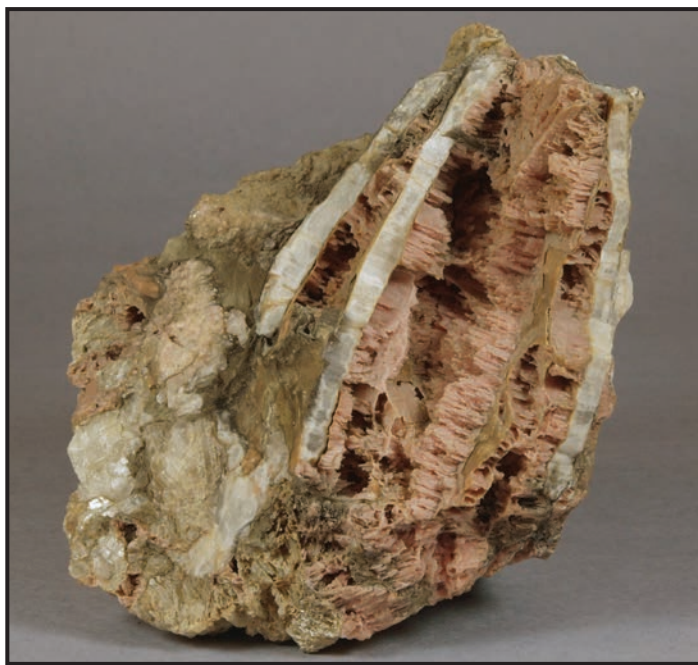
Figure 11. An open breccia from Sterling Hill, containing several generations of calcite. The oldest, the massive white to pale tan material at lower left, is skeletal and strongly etched by solution. The white “ribs” of calcite are probably later. The latest calcite, strongly colored pink, is in parallel plates and needles that collectively form a boxwork texture inherited from some former mineral no longer present. Also present are small masses of a medium-brown, very fine-grained mineral in delicate plumose masses; this resembles todorokite. Franklin Mineral Museum specimen 388, 5.3 × 3.5 × 3.5 inches (13.5 × 9 × 9 cm). Earl R. Verbeek photo.
