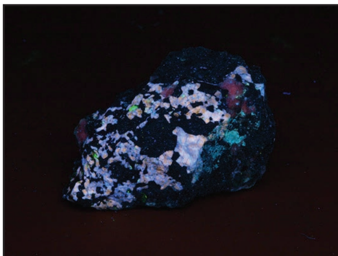
Figure 3b. Mottled pink-and-violet-FL cuspidine under MW UV, with dull red-FL calcite, green-FL willemite, and nonfluorescent franklinite, from the Buckwheat Dump, Franklin, N.J. Compare to Figure 3a. This clearly shows the color shift under MW UV that is a distinguishing feature of Franklin cuspidine. To the eye cuspidine's FL color under MW is usually more violet than pink. Earl R. Verbeek specimen and photo.
