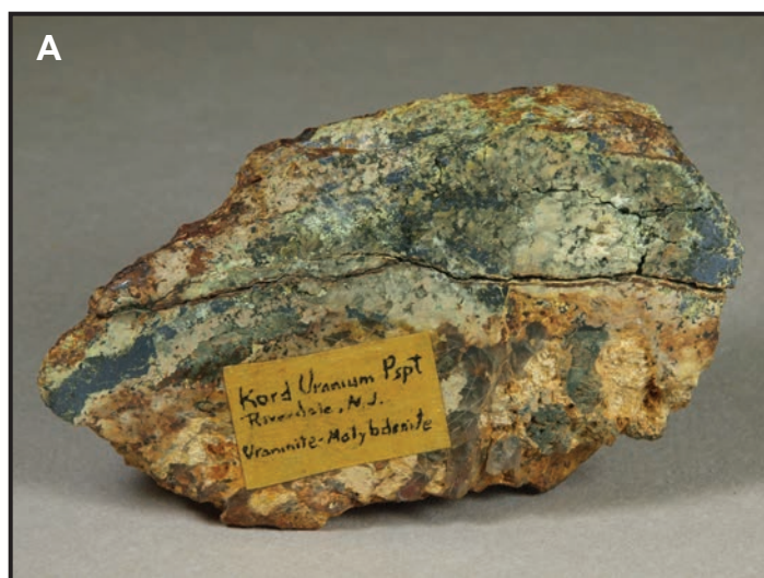
Figure 3. A sawn specimen of uraninite and molybdenite in Precambrian gneiss from the Kord Uranium Prospect, Riverdale, N.J., which was located where the Algonquin Gas Transmission Pipeline crosses Route 23, behind the present-day Pier 1 Imports. Radioactivity is 12 times background at a distance of six inches (15 cm). Under shortwave ultraviolet light, the associated uranyl salts fluoresce bright green. Specimen measures 3.1 × 1.8 × 1.0 inches (8 × 4.5 × 2.5 cm). Franklin Mineral Museum specimen, formerly in the collection of John L. Baum. Earl R. Verbeek photos.
