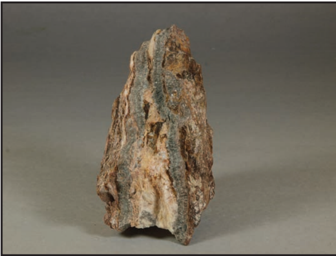
Figure 5. Highly fluorescent and phosphorescent, ivory-colored to pale orange, intergrown columnar grains of willemite with dark brown serpentine and gray dolomite, all part of a well-layered vein sequence from the Franklin mine. Franklin Mineral Museum specimen 7381; 3.5 × 2.4 × 1.6 inches (9 × 6 × 4 cm). Earl R. Verbeek photo.
