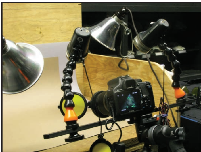
Figure 6. Camera/light configuration for mineral fluorescence photography. Two Sola NIGHTSEA lights are mounted on flexible arms. The barrier filter can be seen swung away from the front of the lens. Two compact fluorescent bulbs in reflectors provide white-light illumination.
