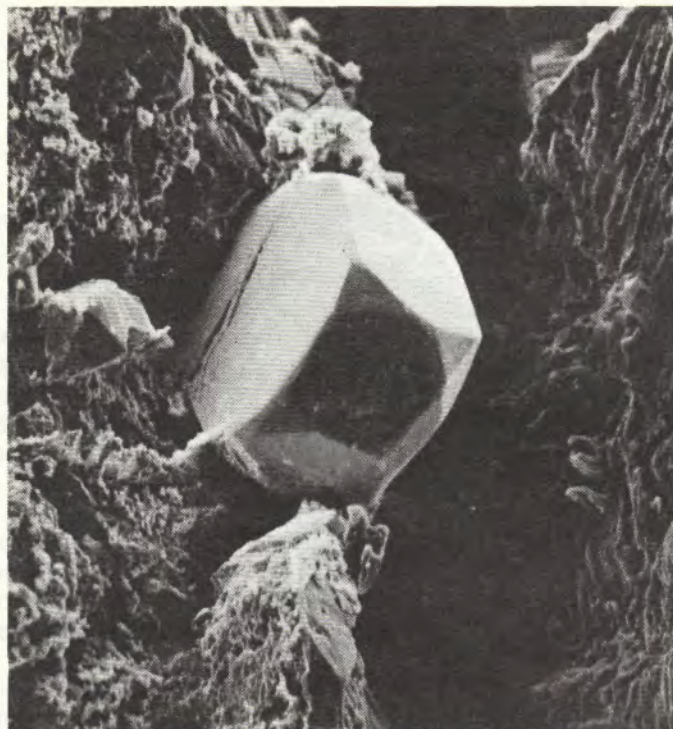
Figure 8. SEM photograph of zircon from Sterling Hill, Ogdensburg, New Jersey. (234X) NMNH #C6101.
