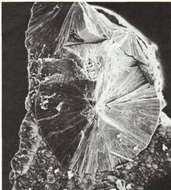
Figure 1. SEM photomicrograph of a cross-section of Sterling Hill austinite showing the radial habit and fibrosity (315X).
