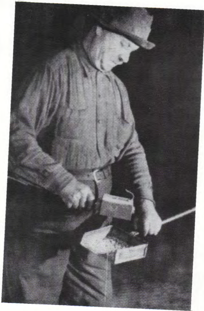
Figure 3. Franklin mill worker viewing fluorescent response of ore concentrate using an early iron arc unit.
