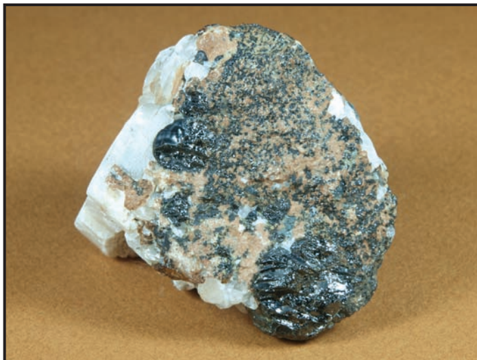
Figure 13. Orange-tan serpentine (probably serpentinized willemite) hosting myriad tiny grains of franklinite in contact with larger grains of franklinite and coarse-grained white calcite. The specimen is labeled Franklin rather than Sterling Hill and measures 6 × 5 × 3.5 cm. Richard Bostwick collection; formerly no. DW721 in the collection of Dru Wilbur.
