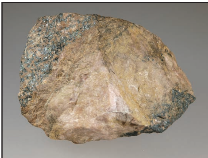
Figure 1. Specimen MB2519. Note the abundant franklinite on either side of a zone of pink grossular and tan feldspar. Maximum width of specimen in this view is 4.1" (10.5 cm). Earl R. Verbeek photo.
