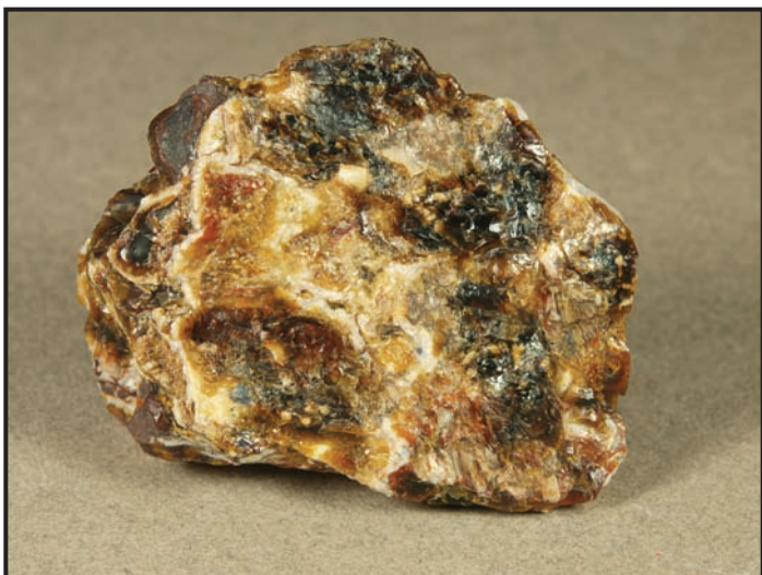
Figure 11. A vein consisting of translucent to locally transparent dark brown serpentine and white calcite, both in thin, irregular layers, upon a matrix (not visible, on back of specimen) of altered granular franklinite-calcite-willemite (serpentinized) zinc ore. The photograph was taken perpendicular to one of the serpentine layers in the vein. The specimen, 5 × 4 × 3 cm, is from the North Ore Body at Sterling Hill. Richard Bostwick specimen, formerly in the Al Smith and “Sunny” Cook collections.
