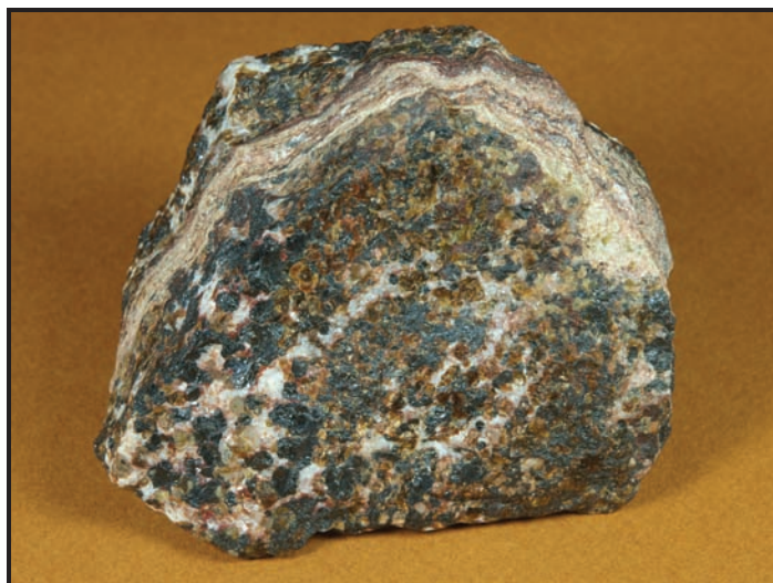
Figure 5. Altered granular ore from the 1750 level at Sterling Hill, consisting of abundant black franklinite, white calcite (stained red by hematite where in contact with franklinite), and abundant honey brown to ochre brown, translucent chrysotile with resinous luster and conchoidal fracture. A layered vein of tan to reddish brown, fine-grained sphalerite cuts the specimen at a low angle to the photographed face. James Van Fleet specimen, 8.5 × 7 × 4 cm.
