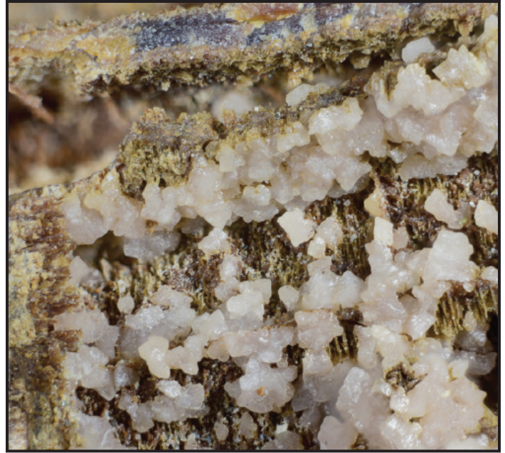
Figure 4b: Close-up view of the tiny (0.5-1.0 mm) rhodochrosite crystals in the specimen of Figure 1. Note that the crystals are nearly white with only a faint blush of pink. Field of view is about 5 mm (0.2 inch) across. Vandall King photo.
