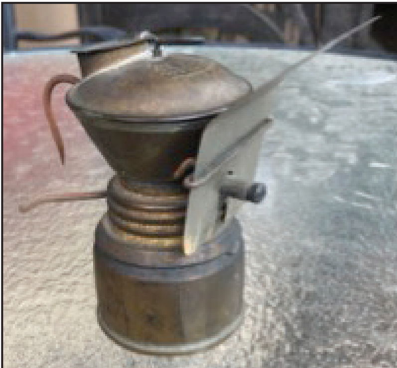
Figures 2-3: A Baldwin carbide cap lamp, showing the wire hook and brace soldered at the back, and a wire brace and removable "wet-mine" reflector at the front. Photos by Dave Thorpe.
