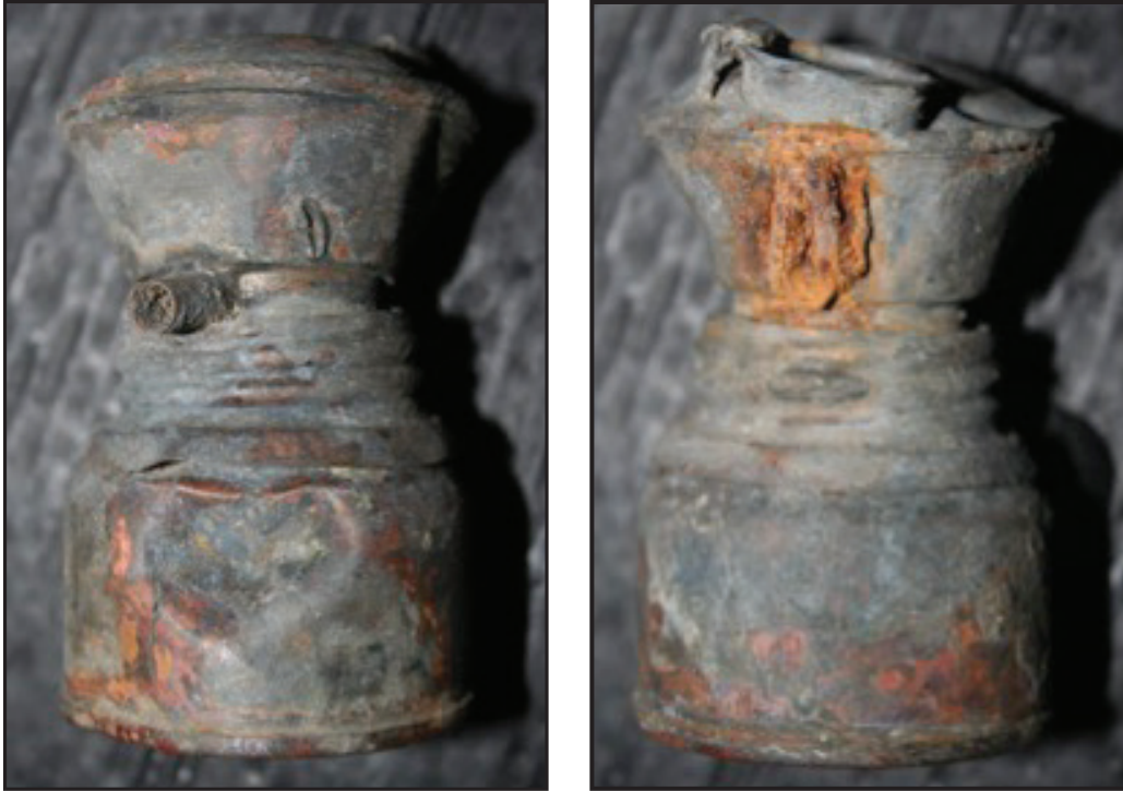
Figures 4-5: Note the solder marks at front and back, the hourglass “pinched-waist,” and the inset water door. The large dent in this lamp bottom made it impossible to maintain a seal between the top and bottom of the lamp, rendering it inoperable. Photos by James Van Fleet.
