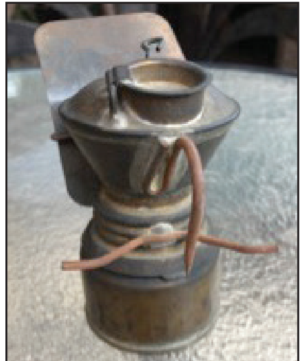
Figures 2-3: A Baldwin carbide cap lamp, showing the wire hook and brace soldered at the back, and a wire brace and removable "wet-mine" reflector at the front. Photos by Dave Thorpe.
