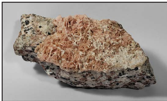
Figure 1: Platelike crystals of pale orange-pink rhodochrosite thickly encrusting a fracture surface in lean, granular, calcite-willemite-franklinite ore. Most of the platy crystals are lying on edge, nearly perpendicular to the fault surface. Lightly encrusting the rhodochrosite in part of the specimen, mostly toward the right, is fine-grained white calcite. Former owners include Richard Hauck, Gary Grenier, and Steven Phillips. Specimen size: 12.8 × 5.3 × 4 cm (5 × 2 × 1.6 inches). Paul Shizume specimen and photo.
